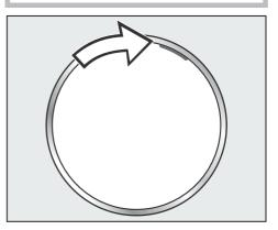
Push the orange marker round to the other side so that you will see at which side to pull the door open.
