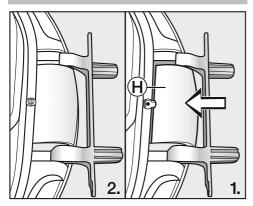
■ Fit new door hinge cover (1) and clip it into position.
