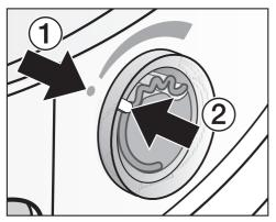
■ Turn the outer ring counter-clockwise until markers ① and ② line up.
