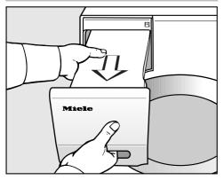
Remove the condensed water container.
