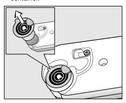
■ Pull out the spout. Remove the spout by holding the side lug and pulling upwards.
