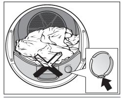
If you are not using a fragrance capsule: The tab must be pushed down completely (see arrow).
