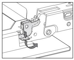
Release the locking clamps on the hinges by pushing them down. Turn them as far as they will go in an angled position.
