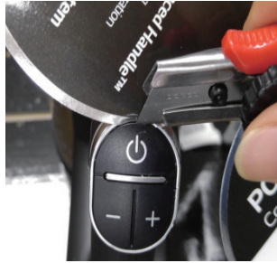
(2) Remove the button with a knife or a sharp object. Use a thick piece of paper in-between to protect the surface of the part, which will have to be replaced if damaged.
