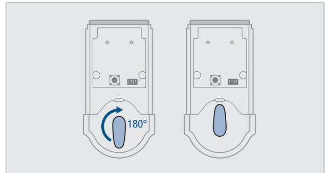
The latch is installed upside down.
