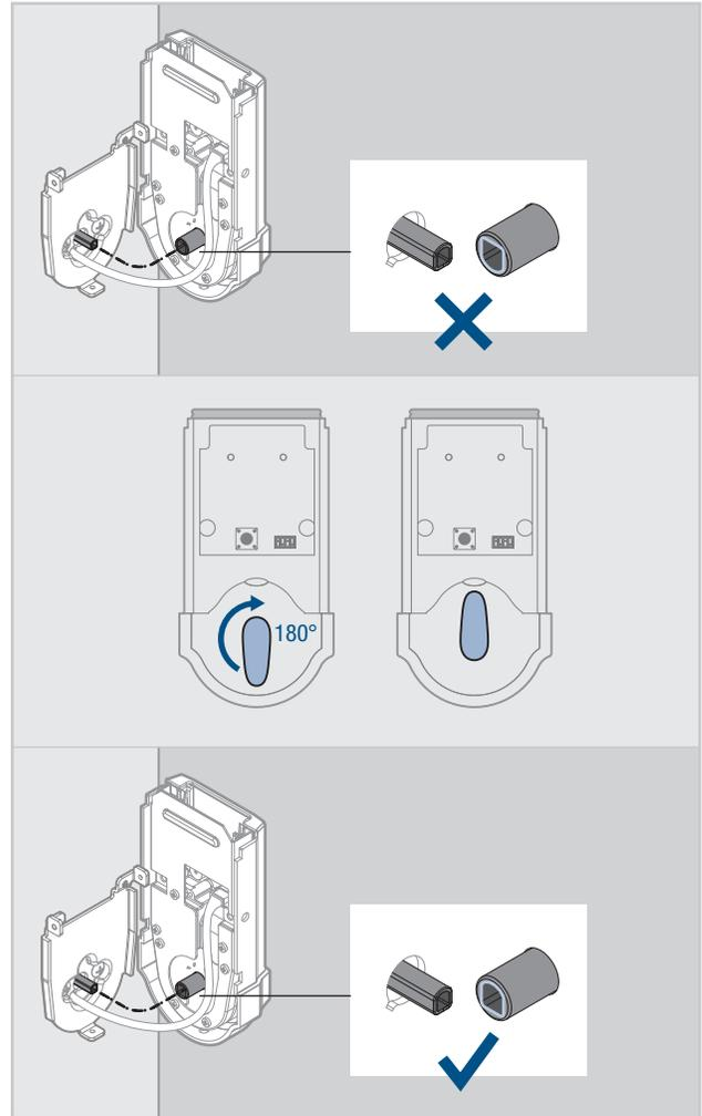
Perform the door handing process once the lock is fully installed.
