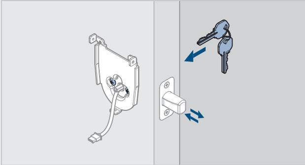
The clutch is disengaged.
