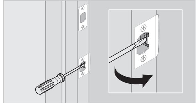
The lower latch and lower strike (for your knob or lever) are misaligned, putting too much load on the deadbolt latch.
